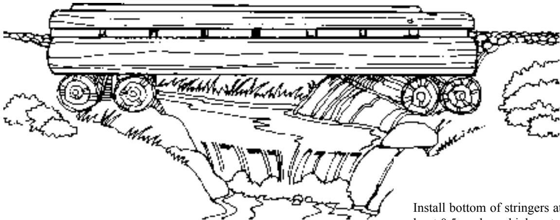
Figure 10.2 Bridge installation with simple foundation details.
