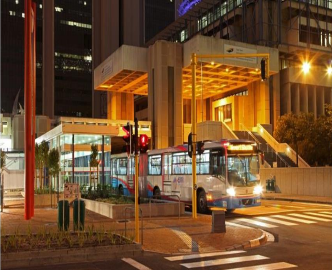
CPT MyCiti main BRT interchange with 18m articulated high floor bus suited for high floor median stations
