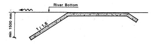
Figure 2 - Section through a typical drift on the Marich Pass – Lodwar road
