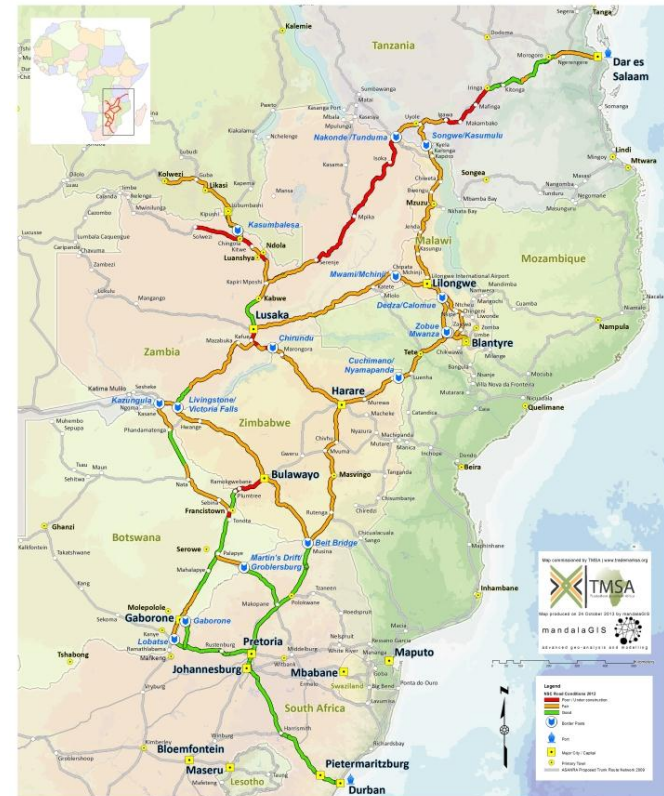
North-South Corridor Networks Road Conditions (as at December 2012)
