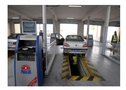
8 lines to verify vehicle components for security reasons and assess pollution level to comply with the standards.
